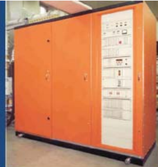
RF power amplifier (Thomson) P_{max} 90 kW CW, Frequency range 15-50 MHz.
