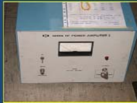
Driver Amplifier (ENI) P_{max} 200 W
